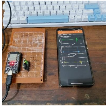
Figure 3. Calibration of the MPU6050 sensor with a smartphone sensor as a reference
