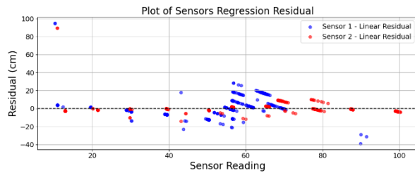
Figure 8. Comparison of two sensors results of characterization process (up) linear regression, (bottom) absolute error plot.
