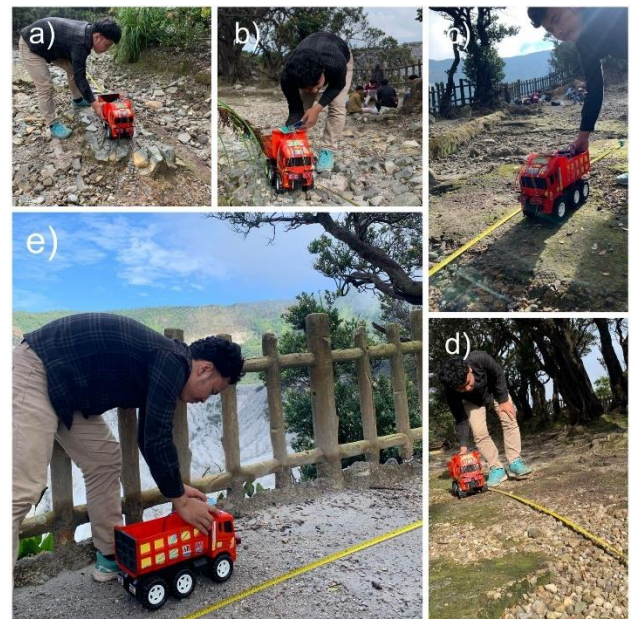
Figure 7. The test fields on the stratovolcanic mountain: a) Rocky inclined surface descending, b) Rocky inclined surface climbing, c) Straight surface, d) Rocky straight surface, e) Sandy road.
