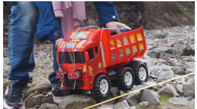
Figure 3. The toy truck as the mobile robot prototype with two ultrasonic sensors.
