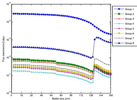
Figure 2. Neutron flux distribution radial axis
