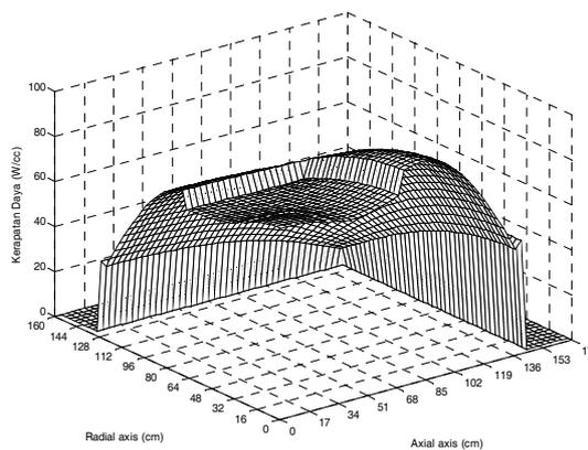
Figure 4. Power density distribution in core
