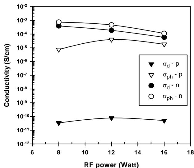
Figure 4. Conductivity of p- and n-layers under RF power discharge optimization: dark conductivity of p-layer ( $\sigma_{d-p}$ ), photoconductivity of p-layer ( $\sigma_{ph-p}$ ), dark conductivity of n-layer ( $\sigma_{d-n}$ ), and photoconductivity of n-layer ( $\sigma_{ph-n}$ )
