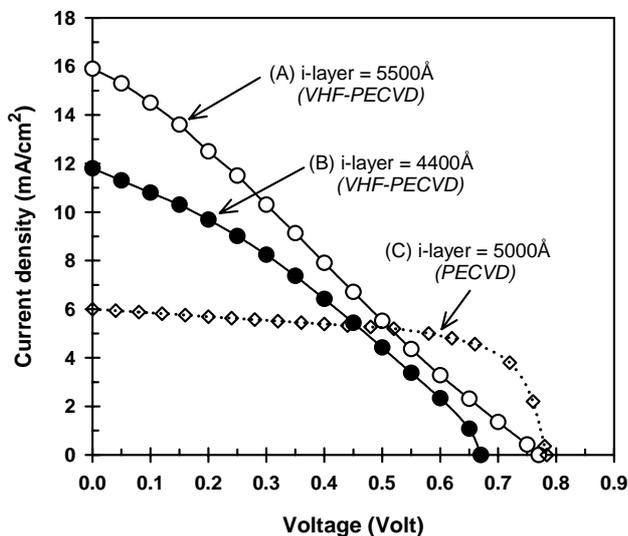
Figure 5. I-V characteristics of fabricated p-i-n a-Si:H solar cells which were resulted from this study using VHF-PECVD (A and B) and from previous study using PECVD (C)
