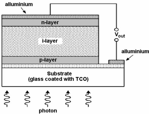
Figure 1. The structure of p-i-n solar cell
