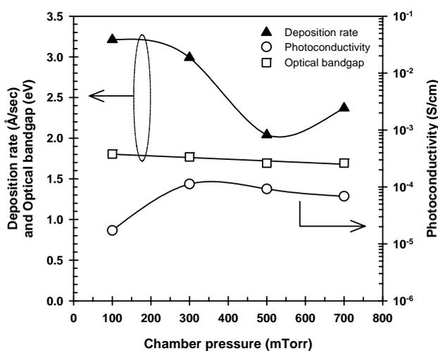
Figure 3. The characteristics of i-layers which resulted under optimization of chamber pressure
