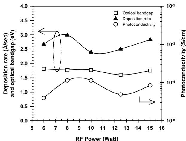
Figure 2. The characteristics of i-layers which resulted under optimization of rf power
