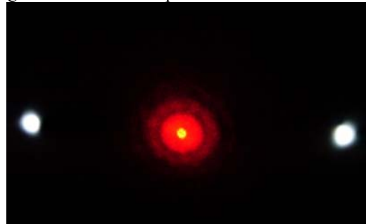
Figure 1. The image of the diffraction pattern for the particles under study using He-Ne laser.
